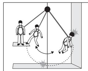
We will ensure as far as it can to focus on work situations with a fall factor 0 or 1 and we will be avoided if possible to install a fall arrest system on an anchor in fall factor 2, the pendulum effect must also be as small as possible.
